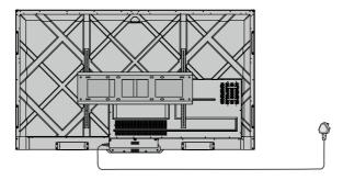
Step 2: Turn on the rocker switch (on the rear side of the screen, next to the power socket) after a power source has been connected. The power indicator should be red.
